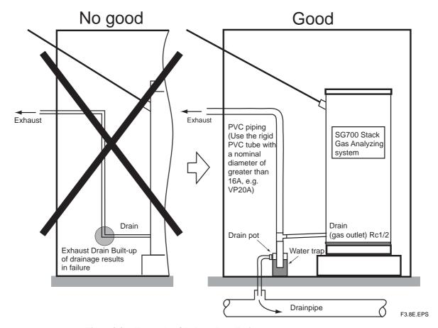
Figure 3.8 Example of Indoor Installation
