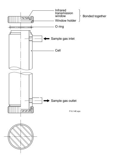
Fig. 10.13 Structure of sample cell (pipe cell)
