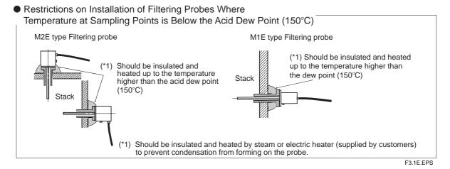
Figure 3.1 Restriction on Installation of Filtering Probes Where Temperature at Sampling Points Below the Acid Dew Point (150 °C)
