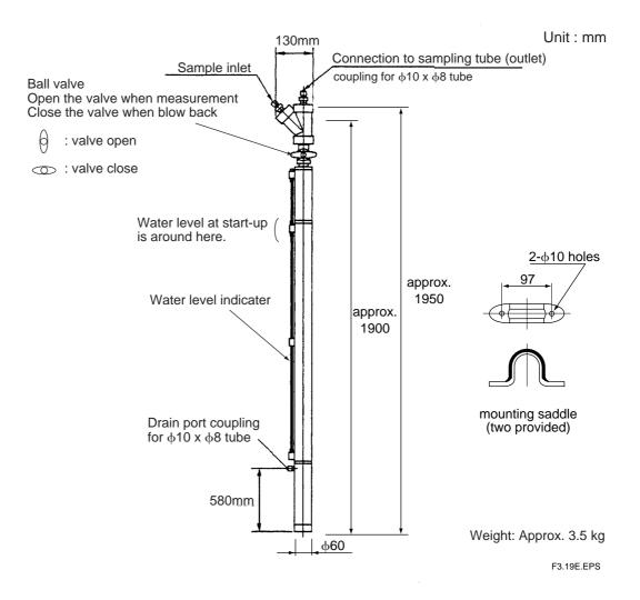
Figure 3.17 Installation of External Drain Separator
