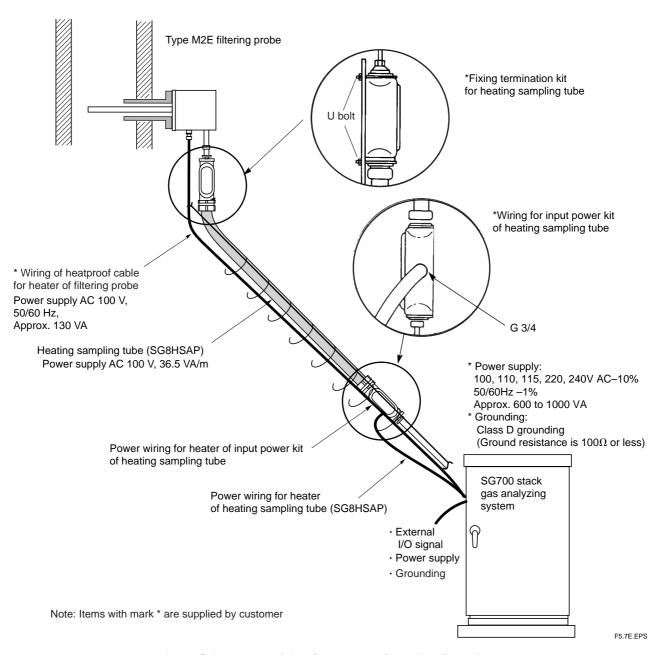
Figure 5.6 Power Wiring for Heater of Heating Sampling Tube
