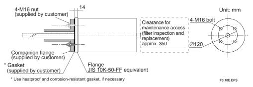
Figure 3.16 Mounting of Types M2E Filtering probes
