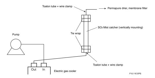
Figure 10.10 Connection of SO<sub>3</sub> Mist Catcher to other devices
