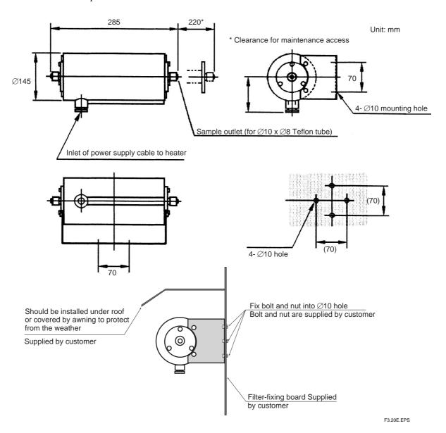
Figure 3.18 Installation Example of Type M1E External Primary Filter
