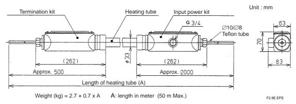
Figure 2.1 Heating sampling tube
