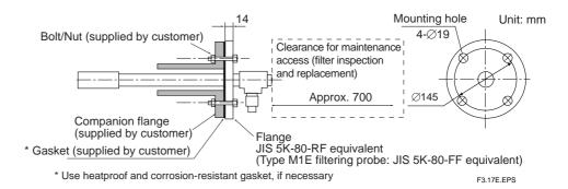
Figure 3.15 Mounting of Types F, M1E, M2 and M3 Probes
