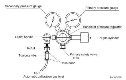
Figure 4.6 Pressure Reducing Valve for Gas Cylinder
