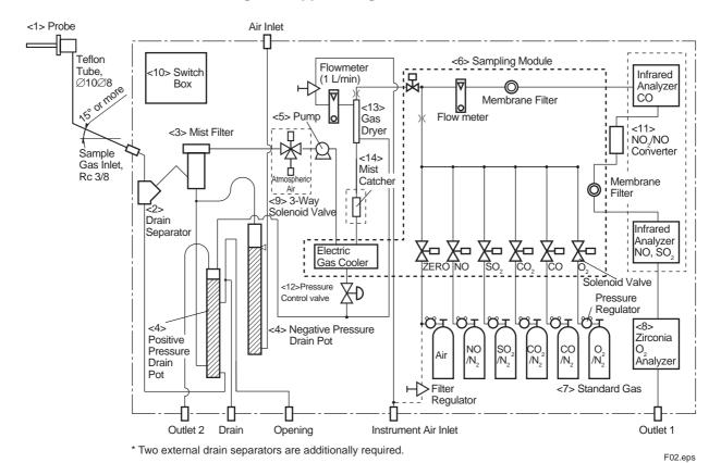
Figure 1.2 Example 2:Five-Component Gas Sampling System Configuration
