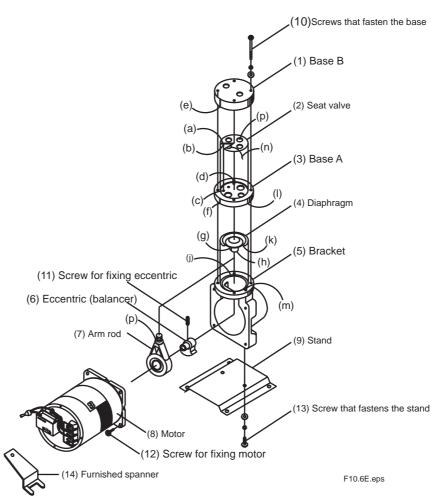
Figure 10.5 Exploded View of Diaphragm-type Aspirator
