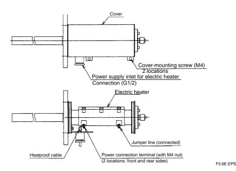
Figure 5.5 Example of Wiring for Filter's Heater
