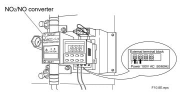
Figure 10.7 Location of NO<sub>2</sub> / NO converter
