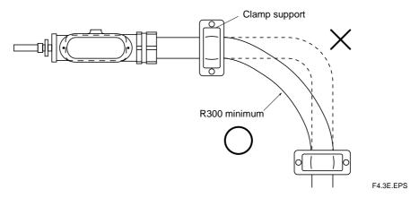
Figure 4.3 Installation of Heating Sampling Tube
