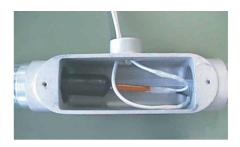
8. Pass the bundle through the connector body (8) on the process piping, the sealing bush (9), washer (10) and nut (11), then securely tighten the bundle-side gland nut.
