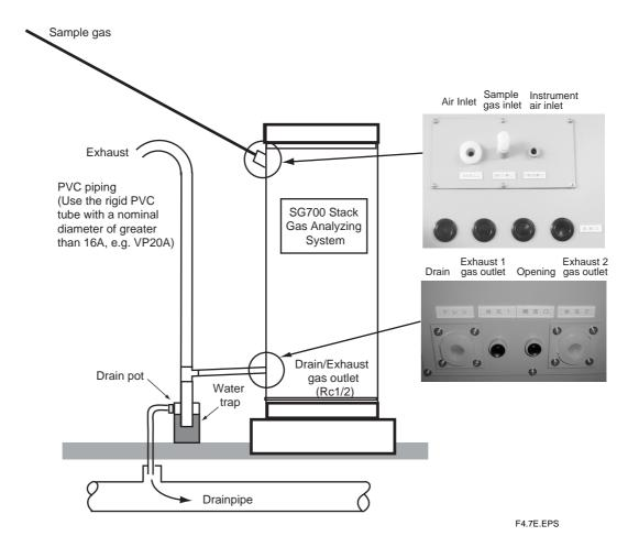
Figure 4.4 Example of Piping for Gas Outlet
