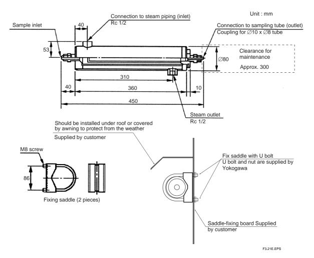
Figure 3.19 Installation Example of Type MS External Primary Filter
