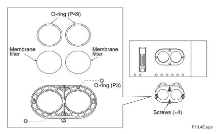
Figure 10.3 membrane filters and their related components
