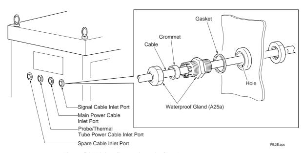
Figure 5.2 Wiring Connections via Glands
