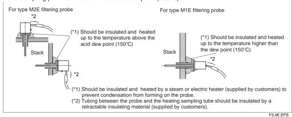
Figure 3.4 Installation Restrictions Where Temperature at Sampling Point is Below the Acid Dew Point (150  $^{\circ}C)$
