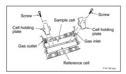
Figure 10.12 Sampling cell and its related parts
