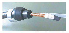
Pass piping bundle through (1) gland nut and (2) sealing bush.
