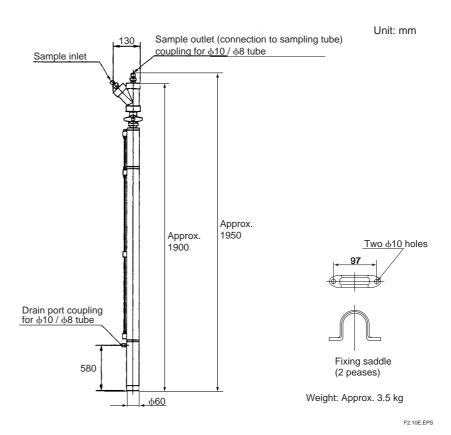
Figure 2.2 External Drain Separator with Safety Trap
