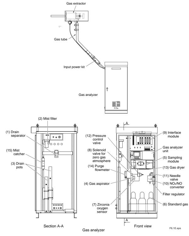
Figure 6.1 Component Names of Devices Inside Front Door (5 components type)
