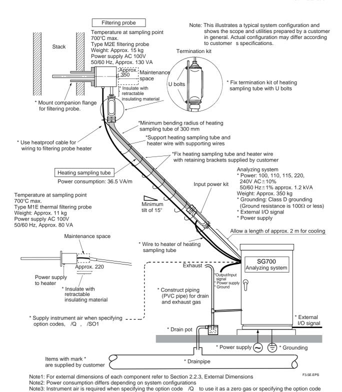
Figure 3.5 Installation of System Using Heating Sampling Tube
