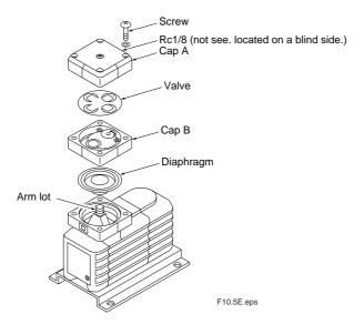
Figure 10.4 Diaphragm type pump
