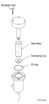
Figure 10.2 Mist filter and its related components
