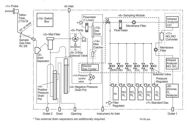
Figure 6.5 Example of Sampling System
