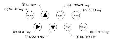
Figure 8.1 Operation Panel (Front View)
