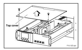
Figure 10.11 analyzer Unit
