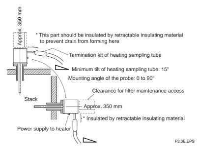
Figure 3.3 Mounting Angle of Type M2E Filtering Probe
