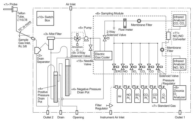
Figure 1.1 Example 1: Five-Component Gas Sampling System Configuration
