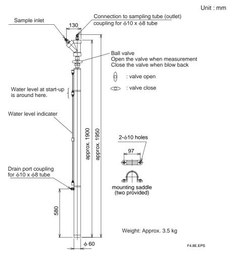
Figure 4.5 Piping for Drain Port of External Drain Separator
