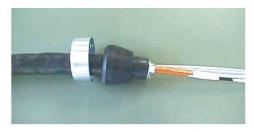
4. Pass piping bundle through (1) gland nut and (2) sealing bush.
