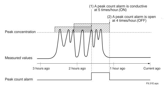
Figure 9. Example of peak alarm action
