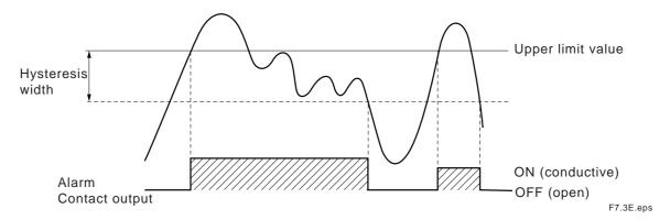
Figure 7.3 Hysteresis (In case-of upper limit Alarm)
