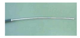
Remove PVC cover and thermal insulation Length to be removed: (200 + L) mm, where L is distance from input power kit to process piping connection.
