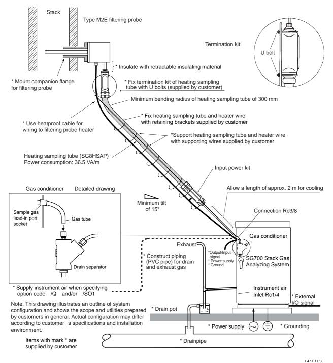
Figure 4.1 Installation of System Using Heating Sampling Tube
