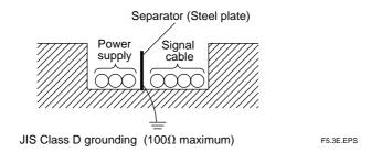
Figure 5.3 Example of Wiring Construction
