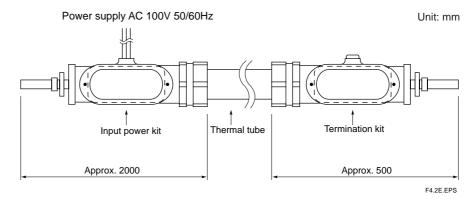
Figure 4.2 Heating Sampling Tube
