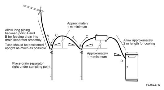
**Figure 3.14 Piping for Sampling** See section 4 for piping procedures
