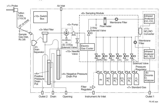
Figure 6.4 Example of Sampling System
