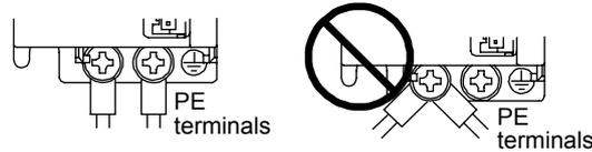
If using an earth-leakage current breaker, always ground the protective earth (PE) terminal of the servo amplifier to prevent an electric shock. Only an RCD (earth-leakage current breaker) of type B can be used for the power supply side of the product.
