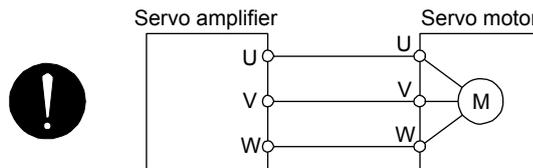
(b) The power supplied to the servo amplifier should not be connected to the power outputs (U, V, and W). Doing so will fail the connected servo amplifier and servo motor.
