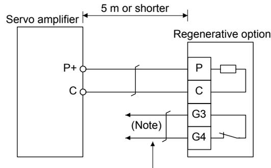
Configure up a circuit which shuts off main circuit power when thermal protector operates.
