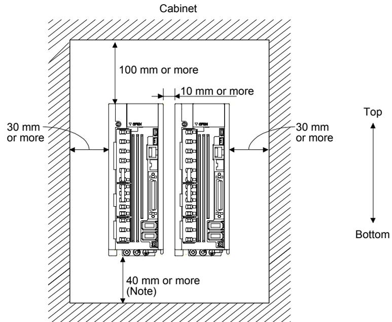
Note. For 11 kW to 22 kW servo amplifiers, the clearance between the bottom and ground will be 120 mm or more.
