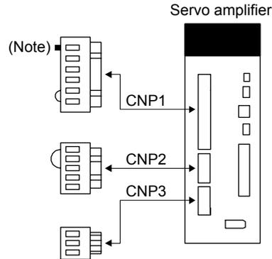
Note. A pin for preventing improper connection is inserted to N- of CNP1 connector.
