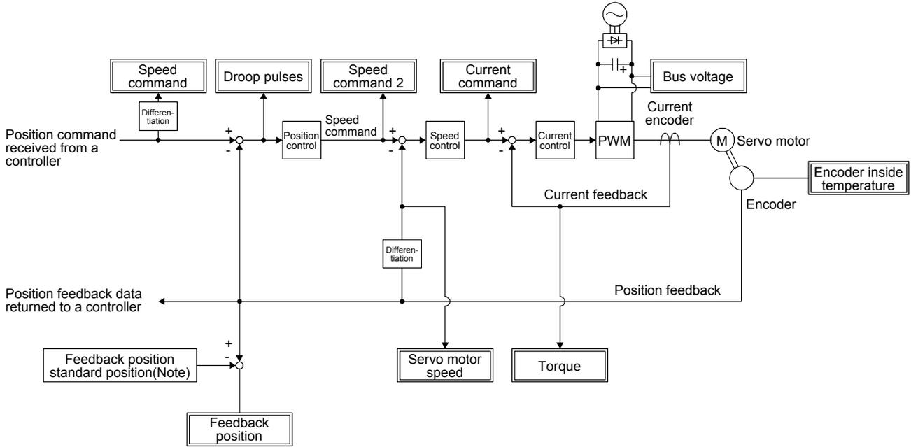
Note. The feedback position is output based on the position data passed between servo system controller and servo amplifier. [Pr. PC13] and [Pr. PC14] can set up the standard position of feedback position that is output to analog monitor in order to adjust the output range of feedback position. The setting range is between -9999 pulses and 9999 pulses.
