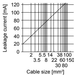
Fig. 9.7 Example of leakage current per km (Ig1, Ig2) for CV cable run in metal conduit
