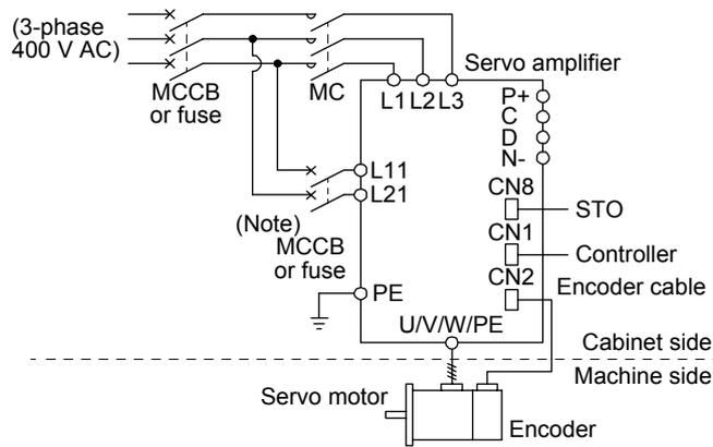
Note. When the wire sizes of L1 and L11 are the same, MCCB or fuse is not required.
