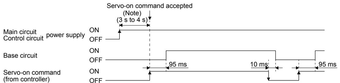
Note. This time period is longer when detecting magnetic pole for the linear servo motor.
