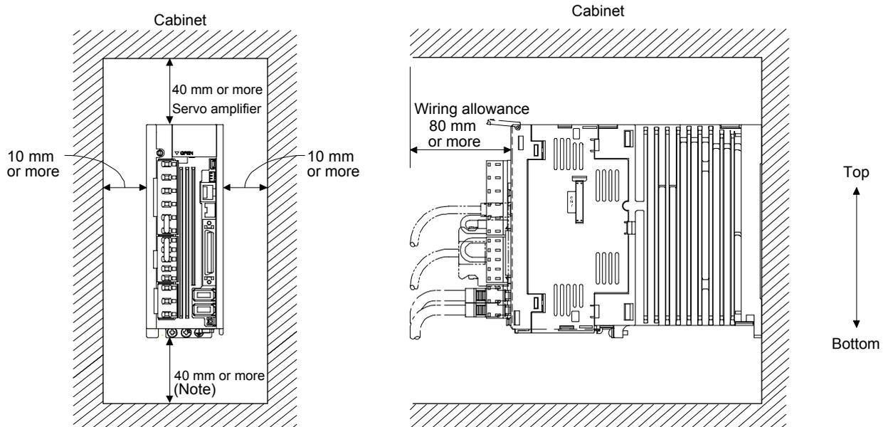
Note. For 11 kW to 22 kW servo amplifiers, the clearance between the bottom and ground will be 120 mm or more.
