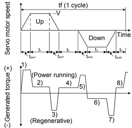
Formulas for calculating torque and energy in operation
