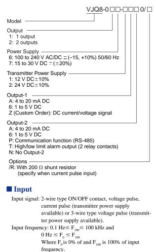
F can be set in increments of 0.0001 (Hz or kHz) within 4 significant digits.
